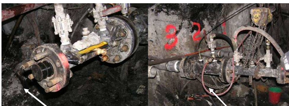
Figure 2: Displacement plug and cement head used during cementing.
